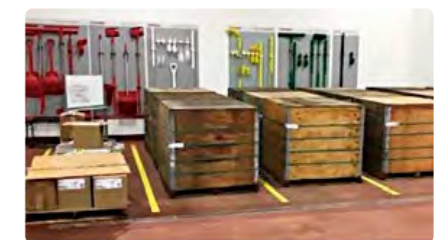
Production floor after Seiri [Sort] and Seiton [Set] in 5S (Kagome Inc. (United States))
